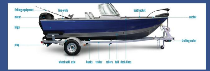
Clean: The hull, below the water line, transom, rear trailer, and watercraft interior
